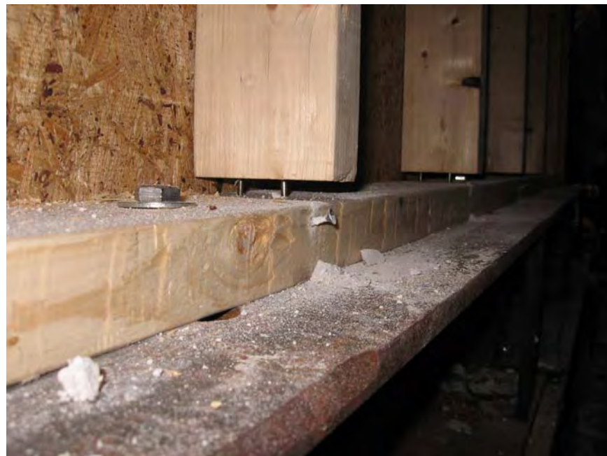
Photo No. 2 Sample #1 Stud Disengagement
