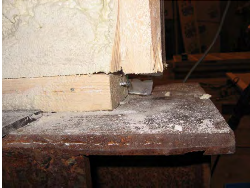
Photo No. 5 Sample #4 Stud Disengagement
