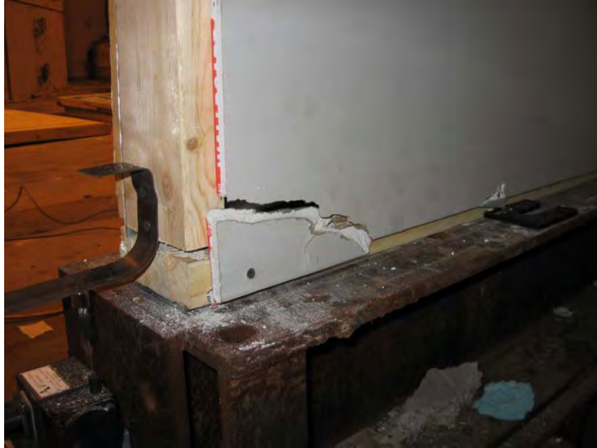
Photo No. 3 Sample #2 Stud Disengagement and Drywall Cracking
